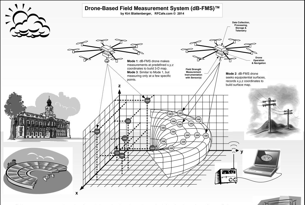
Field measurement space may be outdoors (open air, dense urban, hazardous environment) or indoors (warehouse, theater, factory, office). Drone-based sensors may measure RF/microwave field levels (radio, radar, wireless), acoustic levels (human hearing realm and beyond), light levels (visible, infrared, ultraviolet), subatomic particle levels, gas levels, particulate levels, etc. Directional or non-directional sensors can be used.
