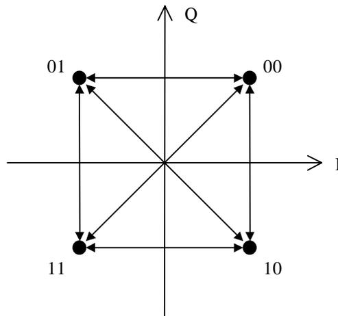
The symbol rate is the bit rate divided by the number of bits per symbol, given by equation (1). The symbol rate for QPSK is one half the bit rate. Twice as much information can be carried with QPSK modulation as compared to BPSK modulation, which has a symbol rate equal to the bit rate. Compared to BPSK, the required channel bandwidth in QPSK for a data rate of 24 kb/s is nearly 100 kHz—an improvement by a factor of two in bandwidth efficiency.
