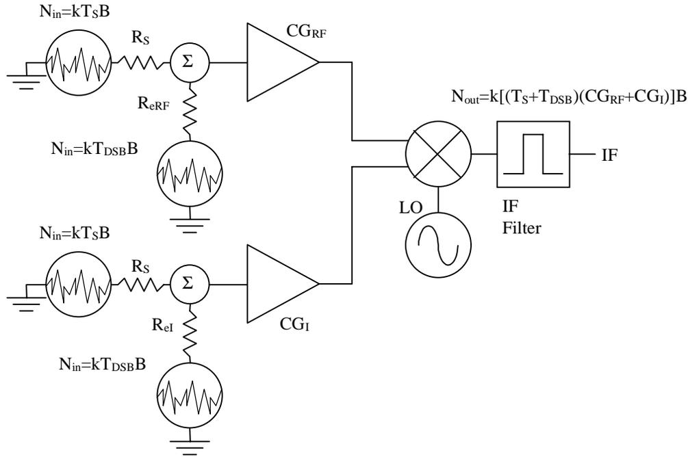
An RF filter in front of the mixer rejects noise in the image band, thus eliminating the need to consider SSB versus DSB noise response. In this case, the mixer SSB NF is used in system budget analysis.
