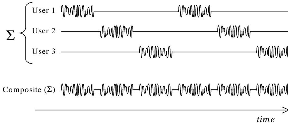
TDMA is sometimes combined with time division duplex (TDD) or frequency division duplex (FDD). With TDD, half of the frame's time slots are used for transmission and half are used for reception. With FDD, different carrier frequencies are used for TDMA transmission and reception, even though similar time slots may be used for both functions.
