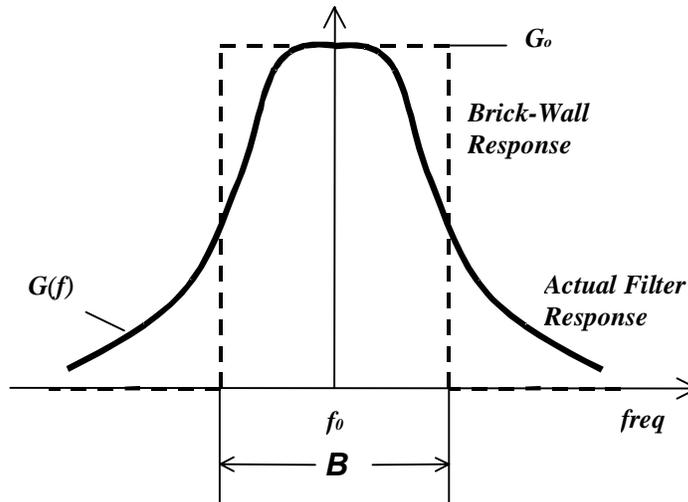
The area under the filter response curve is found by integrating the filter transfer function (response) as a function of frequency and then dividing by the maximum gain  $G_0$  at frequency  $f_0$  using equation (12). The integrand gives the equivalent noise bandwidth to the brick-wall response (see Figure 15).
