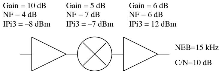
Now, all dB values of gain, noise figure, and input intercept point are converted to numeric using numeric equations. (The last stage gain does not need to be converted to numeric for the cascaded noise figure or cascaded intermodulation distortion equations.) The system numeric gains are given by:
