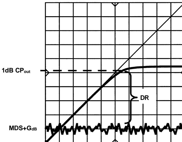
Dynamic range is calculated by subtracting the MDS from the 1-dB compression point referenced to the input. In equation form:
