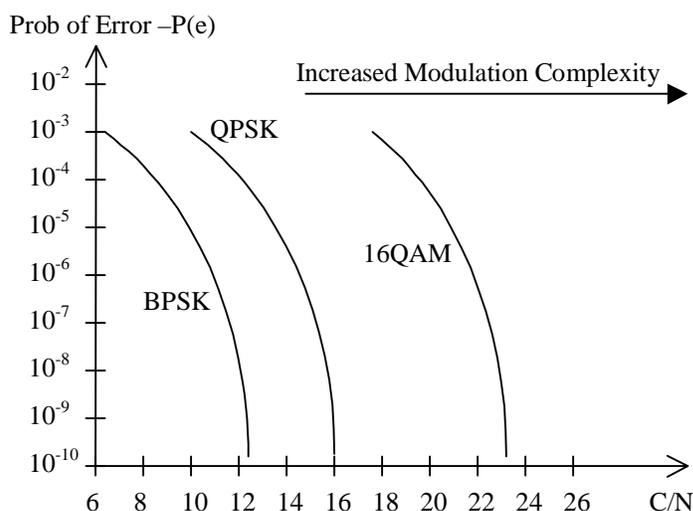
Figure 33 shows the probability of error versus carrier-to-noise ratio for various modulation schemes. BER has a nonlinear relationship to the receiver’s MDS. The higher the desired signal is above the noise floor, the lower the BER ( $P(e)$ ). As signal-to-noise ratio decreases, the probability of error increases dramatically. BER changes by several orders of magnitude with small changes in the signal-to-noise ratio. Consequently, the message reliability decreases with a decreased signal level.
