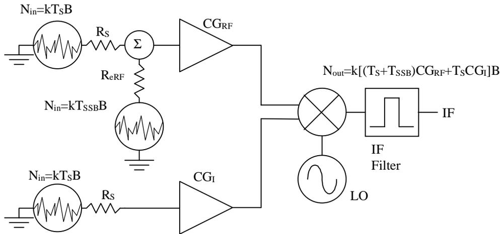
$$(66) \quad N_{out} = k[(T_s + T_{SSB})CG_{RF} + T_s CG_I]B$$
