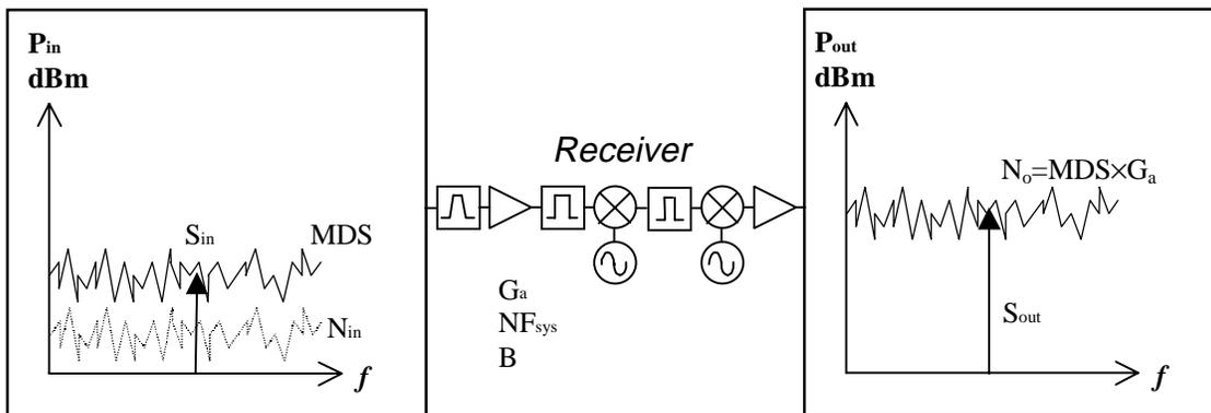
The input referenced noise floor is calculated by subtracting the system gain in dB from the output noise power, thus giving equation (73).
