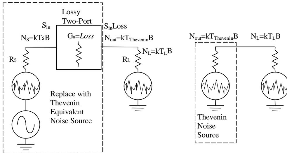
$$(56) \quad G_a = \frac{S_{out}}{S_{in}} = \frac{S_{in} Loss}{S_{in}} = Loss$$
