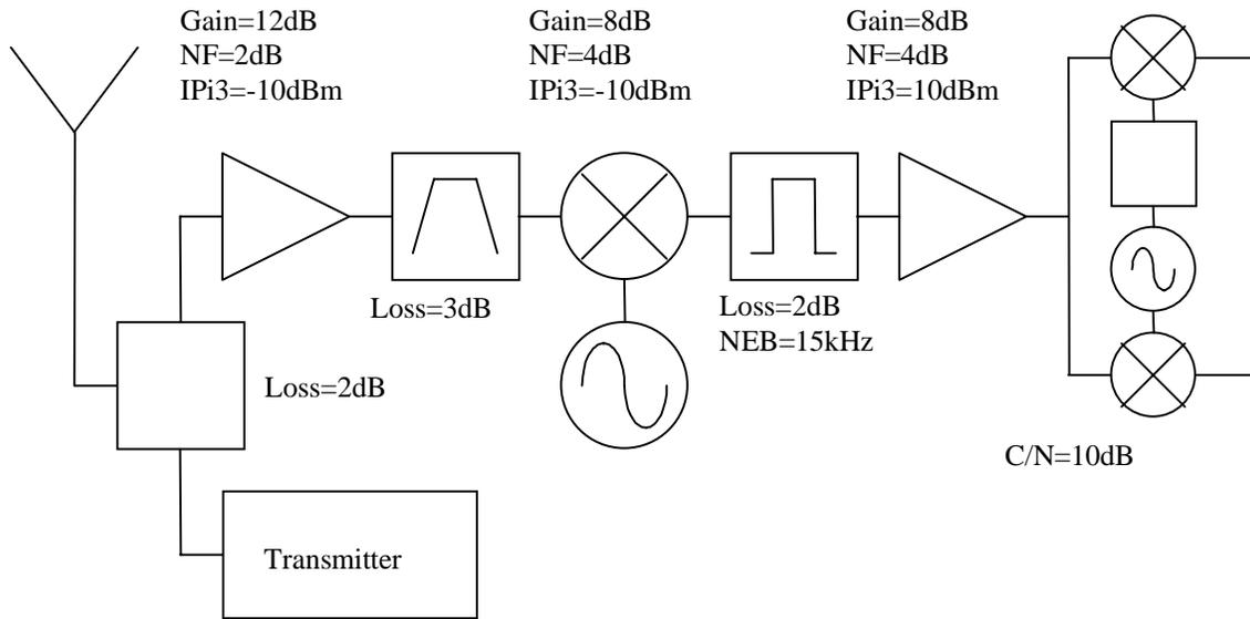
First, the total gain for the system  $G_{\text{sys}}$  is calculated by simply adding all the gains of each stage together.
