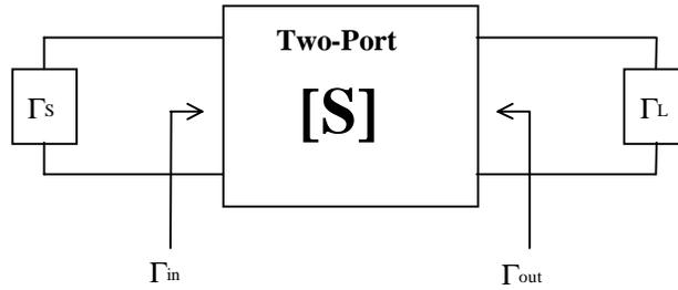
Available gain factor depends on the source termination  $\Gamma_S$  and the s-parameters of the two-port, as shown by equation (18). Available gain dependence on  $\Gamma_S$  may cause two-port mismatch at the input. Available gain depends on the two-port output being conjugately matched to  $\Gamma_L$ ; thus,  $\Gamma_L = \Gamma_{out}^*$ .  $\Gamma_{out}$  is a function of  $\Gamma_S$  and the two-port s-parameters shown by equation (20).
