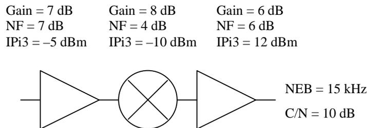
The new sensitivity and spur-free dynamic range are -114.93 dBm and 71.67 dB. Both sensitivity and SFDR were degraded by moving the RF filter.
