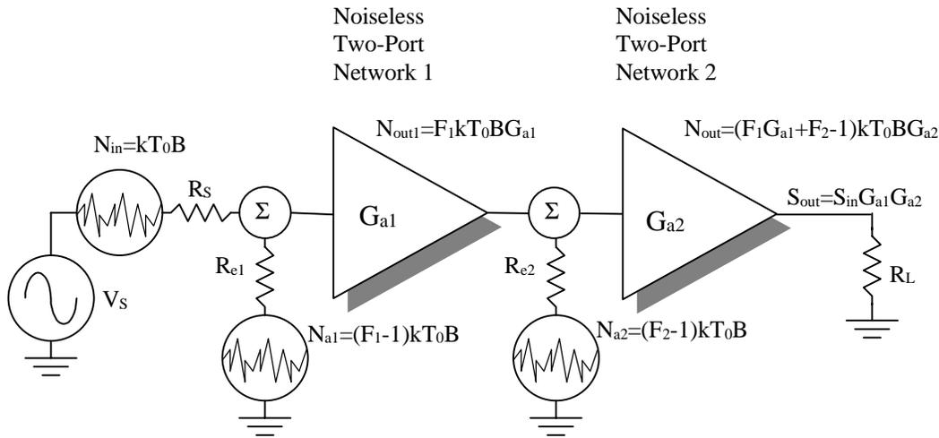
$$(47) \quad N_{\text{out}} = F_1 kT_0 B G_{a1} G_{a2} + (F_2 - 1) kT_0 B G_{a2} = (F_1 G_{a1} + F_2 - 1) kT_0 B G_{a2}$$
