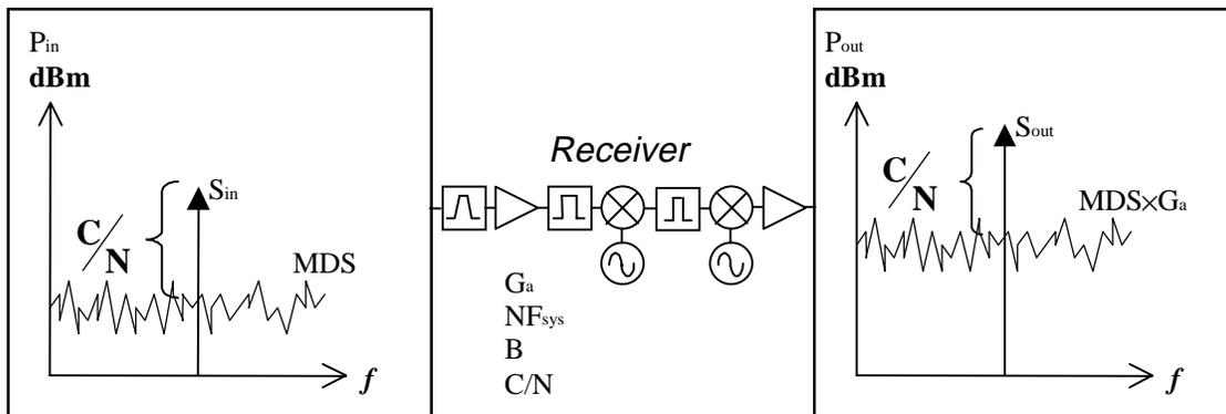
MDS references source noise and noise added by the receiver to its input terminals. This is not the “true” noise floor but a “fictitious” noise floor due to noise added by the receiver. The “true” noise floor is simply the source noise given by equation (74) for  $N_{in}$  ( $kT_0B$ ) when the receiver is terminated by a passive termination at its input. (Figure 31 shows  $N_{in}$  and MDS at the input of a receiver.)
