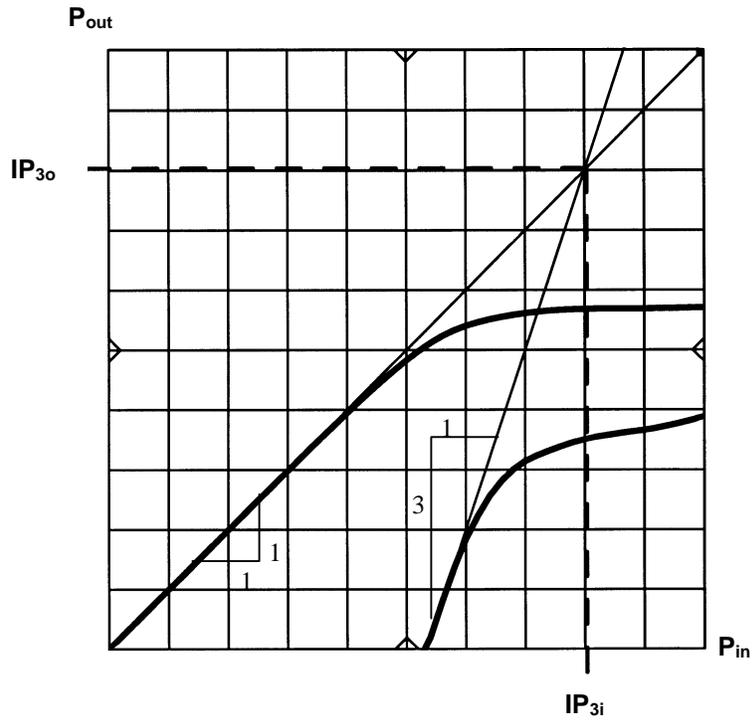
The intercept point permits a full description of the third-order intermodulation distortion as long as the two-port is not compressed. Simple linear relationships allow determination of distortion product power for a given fundamental input or output power level.
