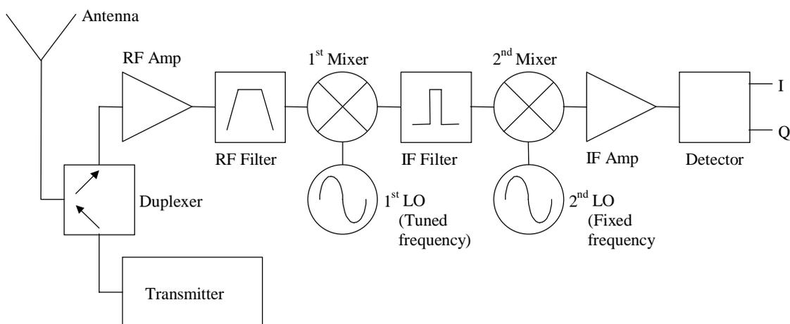
Narrow-bandwidth passive IF filtering is typically accomplished using crystal, ceramic, or SAW filters. These filters offer better protection than the zero-IF receiver gyrator filters against signals close to the desired signal because passive filters are not degraded by the compression resulting from large signals. The active gyrator circuit does not provide such protection. However, the price for improved protection is larger physical size and required printed circuit board real estate.
