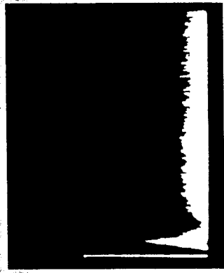
Figure 21A. Noise floor vs. frequency; 0.05 \mu\text{f} decoupling.
