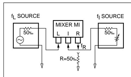
The amount of signal passing through the mixer from the L-port to the R-port is determined by the dc control current present at the I-port. Maximum attenuation is
