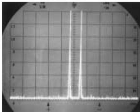
High drive: With a +27 dBm fL drive level, a high power mixer virtually eliminates all two-tone products from the 60 dB spectrum.
