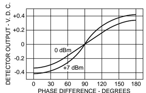
Typical Phase Detector Output vs. Phase Difference
