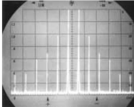
Low drive: With a +7 dBm fL drive level, a balanced mixer can suppress many of the two-tone spurs. However, a number of relatively unsuppressed products remain
