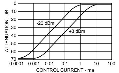
Typical Attenuation vs. Control Current
