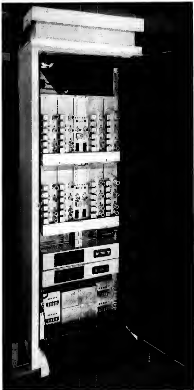
Fig. 37—Typical arrangement of pole mounted repeaters.
