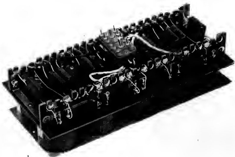
Fig. 32—Typical directional or auxiliary band filter—internal view.
